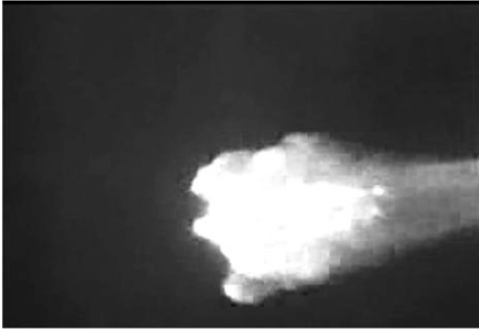
Image 6. Frame 193. A rapid narrowing of the exhaust fumes behind the rocket.
